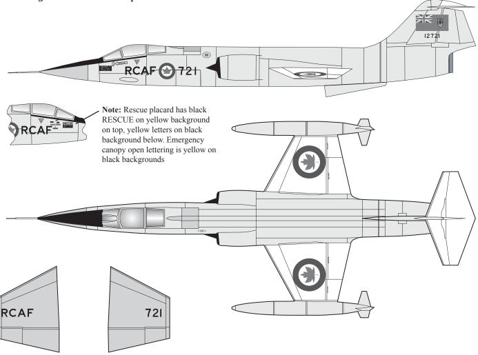
Underside of wings: Note natural metal leading edge strip on top and bottom (horizontal stabs as well)
