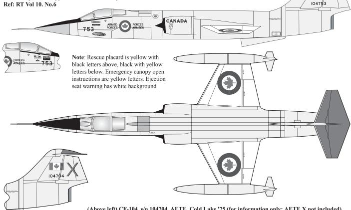
(Above left) CF-104, s/n 104704, AETE, Cold Lake '75 (for information only; AETE X not included) The Central Experimental and Proving Establishment (CEPE) received five CF-104s (12701-05) and one dual (12652) for simulator acceptance and weapons testing. This unit later became Aerospace Engineering and Test Establishment (AETE), and its aircraft carried the red X on the tail. Otherwise, the marking scheme was identical to scheme 6.
