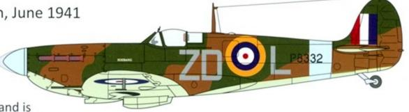
preserved in Canada, the only presentation Spitfire remaining. In June 1941 it was equipped with a Mk I deHavilland propeller and fishtail exhausts. In its preserved state it now has a Mk V Rotol propeller and straight exhaust pipes. We recommend making a Mk IIb by starting with a Vb and modifying the exhausts and propeller to suit. Colours are Dark Green and Dark Earth over Sky, with a Sky Blue spinner and fuselage band.
