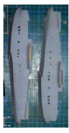
When preparing the fuselage all that really needs to be done is to ensure the mating surfaces are flat.
