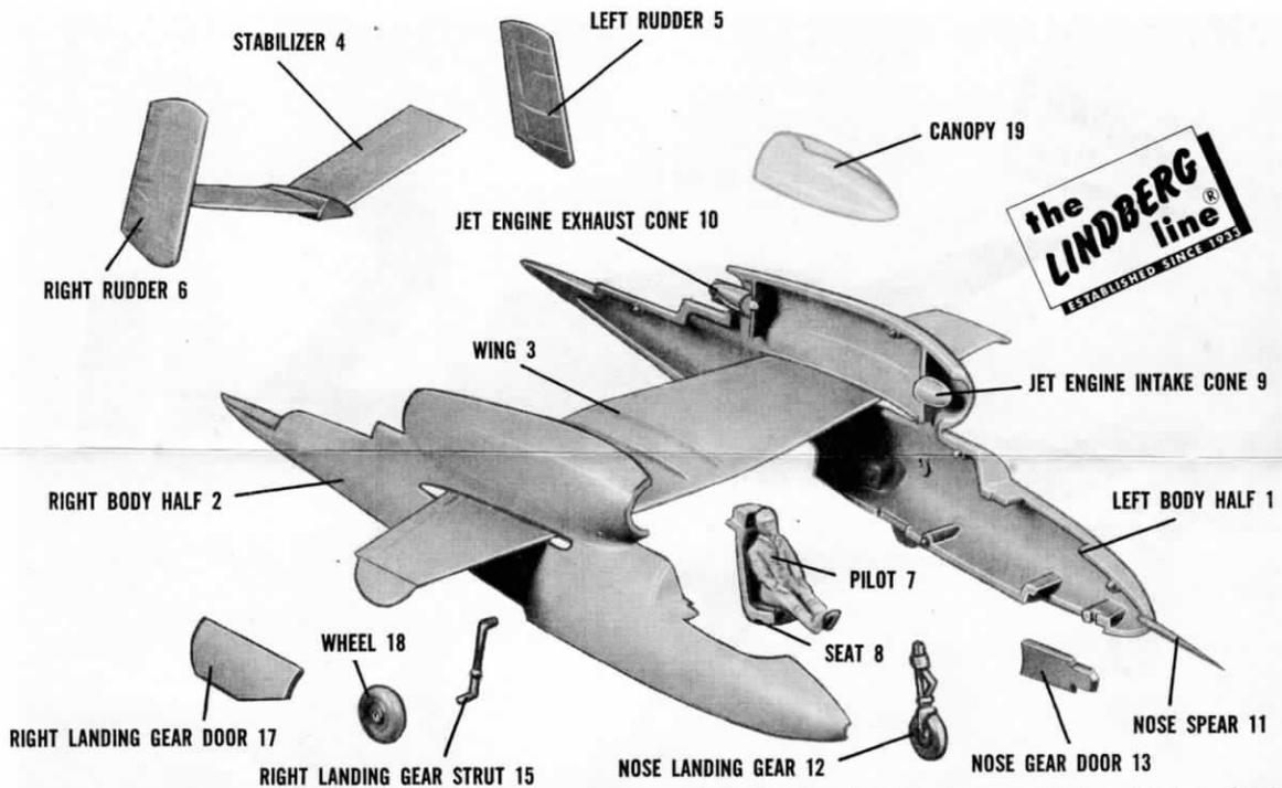
Cement parts 7 and 8 together then into part 1. Cement 9 and 10 to 1. Next place 3 into slots in 1 and 2 then cement 1 and 2 together. Now cement 5 and 6 to part 4 then cement this assembly to body. Cement parts 14, 15, 18, 13, 12, 16 and 17 to body. Finally cement 19 and 11 in place. Cement stand parts 20 and 21 together and place model on stand. See finished picture.
