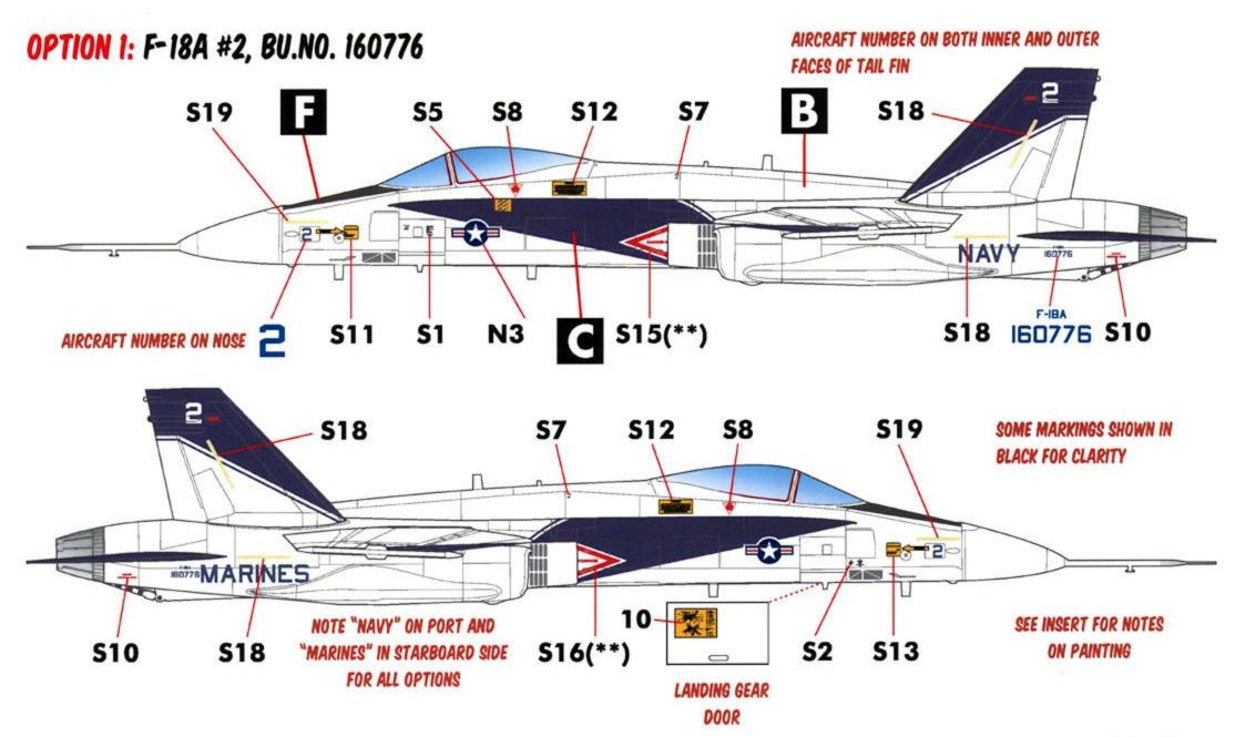
COMMON MARKINGS AND STENCILLING WAS SIMILAR FOR ALL PROTOTYPE HORNETS. USE THIS DIAGRAM FOR ALL OPTIONS ON THIS SHEET. (\*\*): THERE WERE TWO DIFFERENT KINDS OF INTAKE WARNING MARKINGS. ONE OF THEM IS SHOWN HERE - SEE INDIVIDUAL OPTIONS FOR APPLICABLE INTAKE WARNING TYPE.
