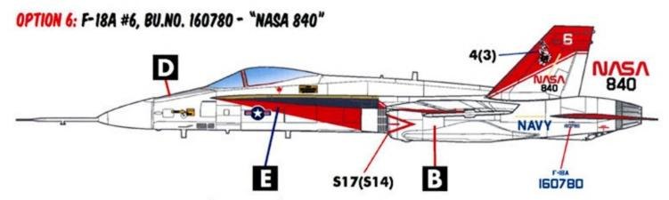
F-18A #6 EVENTUALLY BECAME "NASA 840". BEFORE IT WAS COMPLETELY REPAINTED IN A PROPER NASA COLOR SCHEME, IT MAINTAINED ITS PROTOTYPE COLOR SCHEME; BUT RECEIVED A GRAY ANTI-GLARE PANEL, A NASA LOGO ON THE TAIL, AND SOME FUSELAGE PANELS FROM OTHER F-18A PROTOTYPES. PLEASE VISIT THE REFERENCE SITE FOR THE PHOTOS WE WERE ABLE TO FIND.
