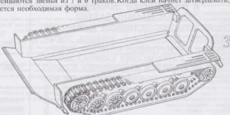
Catepillars are assembled of links made of 4,5,6,7,21, and 23 tracks. First glue the links of 23, 21, 4, and 5 tracks and only then the link of 7 and 6 tracks. When the glue begins to harden, shape the caterpillar.
