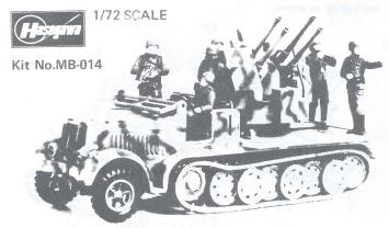
Based on the design of the very successful prime mover Sd.Kfz 7, the 7/1 was modified to mount the German 2 cm Flakvierling quad 38 anti-aircraft gun. Having a rate of fire of some 800 rounds per minute and a range of two miles, the quad 38 made a very formidable anti-aircraft weapon.
