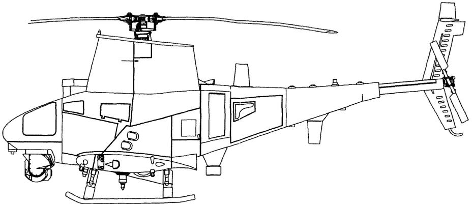
The MQ-8B helicopter was developed as part of the VTUAV (Vertical Take-off UAV) programme commenced in 2000. The helicopter, as a drone, is going to be an excellent tool for use from small ship decks, and when used on land it requires no airfields and can be used from unprepared fields. The feature will allow, apart from reconnaissance duties, to use these machines to deliver supplies to fighting troops. Design of the machine is derived from the Schweizer 333 two-seat civil helicopter.
