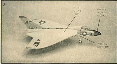
You may attach the decals without painting the model. It is more realistic to paint the model however. Apply the decals as shown here and on the four-view plan.
