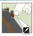
Glue the chimney top into position. Once the glue has set use the supplied guide marks to a drill hole for a chimney pot (not supplied). Chimney pots can easily be created by painting any tubing of a suitable diameter (for example, brass, styrene, ballpoint ink tubes or cotton buds) a red brown colour. Alternatively commercially available pots can be used.
