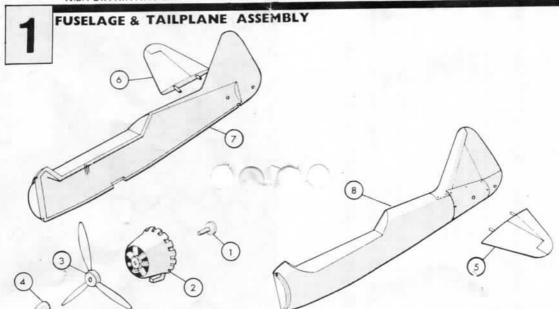
It is recommended that the instructions and exploded views are studied and the assembly practised before cementing together. If it is wished to paint internal details such as crew and cockpit interior this is best done before assembly.
