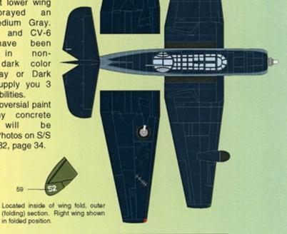
AIRCRAFT 6 • Eastern (Grumman) TBM-3D Avenger, VT(N)-90. USS Enterprise (CV-6), March 18/19, 1945. Non-Specular Sea Blue uppersurfaces with Intermediate Blue vertical surfaces. White undersides oversprayed with dark color, possibly Non-Specular Sea Blue or Intermediate Blue. Black is also a possibility. White propeller boss and wheels.
