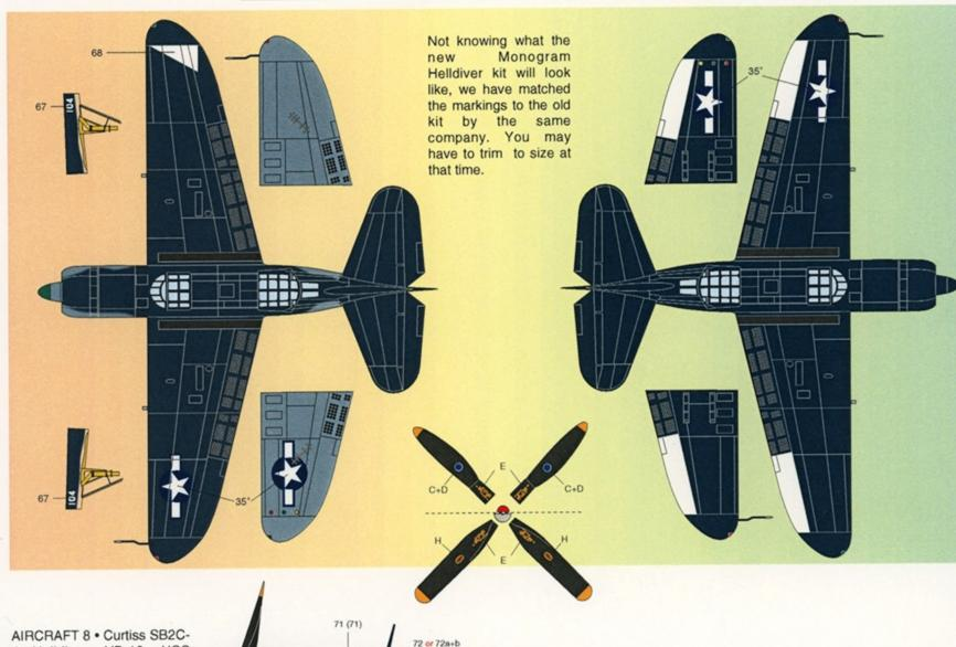
AIRCRAFT 8 • Curtiss SB2C-4 Helldiver, VB-12, USS Randolph (CV-15), February 17, 1945. Overall Gloss Sea Blue. Aircraft was fitted with rocket stubs.
