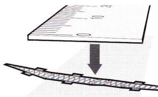
Place a flat edge object like a ruler on the Etched parts.
