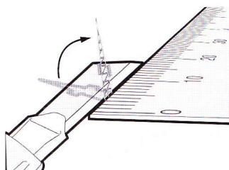
Place the knife under to bend, and carefully lift the side of the knife to fold the etched parts.
