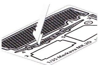
Cut off Photo Etched parts using a utility knife carefully.
